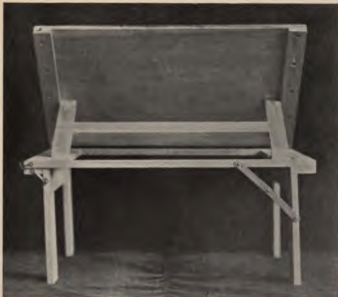
Fig. 35.—Bed Table, II. At the right the leg is braced with a modified jack knife desk rest, on the left by a hook. The smaller hook just above it holds the frame and the top together when folded.
